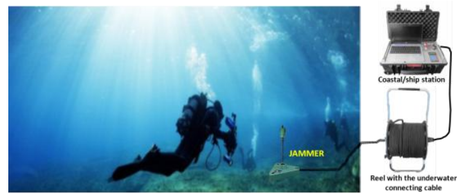
Fig. 4. Composite underwater communications jammer RACK-CS
