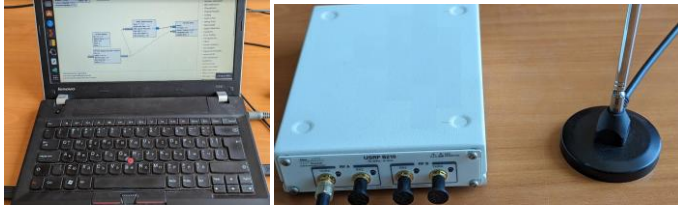
Fig. 6. A structural view of the developed prototype of a software-defined scanning radio receiver for spectrum monitoring and control
