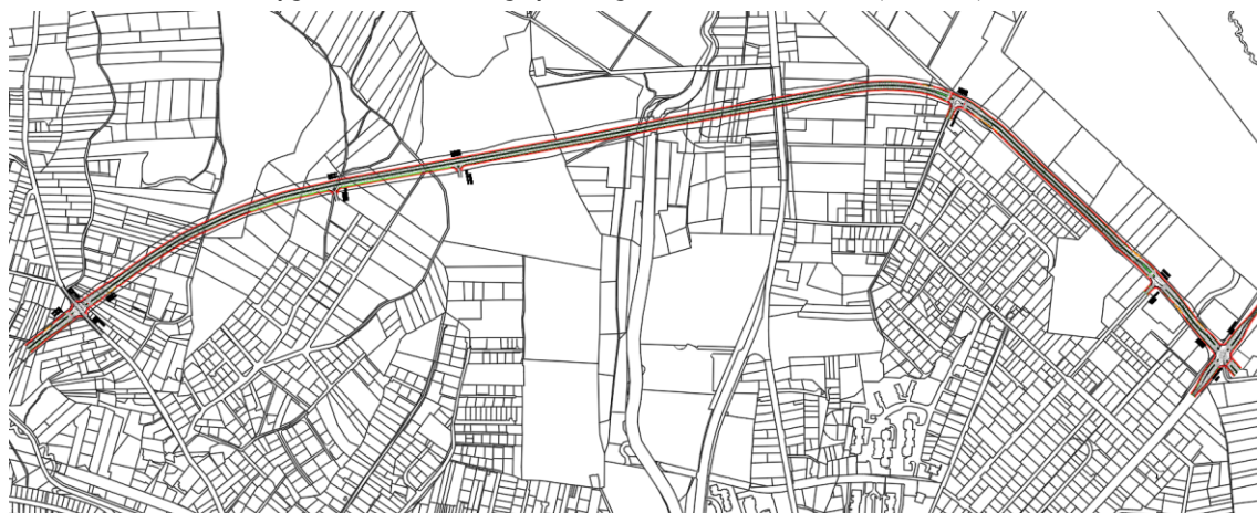
fig. 5. Variant 2 — GUP design with two additional local junctions (AutoCAD).
