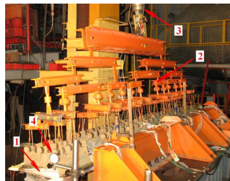
Fig. 5. The aileron on test plant a strain gauge on the shock absorber rod mirror of 1 – Aileron, 2 – Load stand, an aircraft landing gear strut 3– Load hydraulic cylinder, 4 – Indicator
