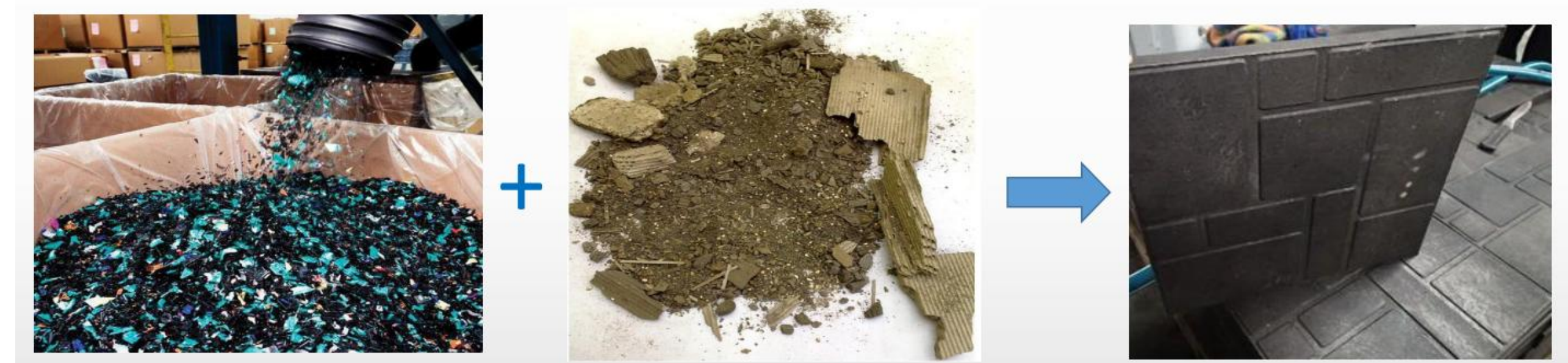
Fig.1. Idea of solution for manufacturing products from polymer-mineral composition; polymer recyclate + mineral filler = product.
