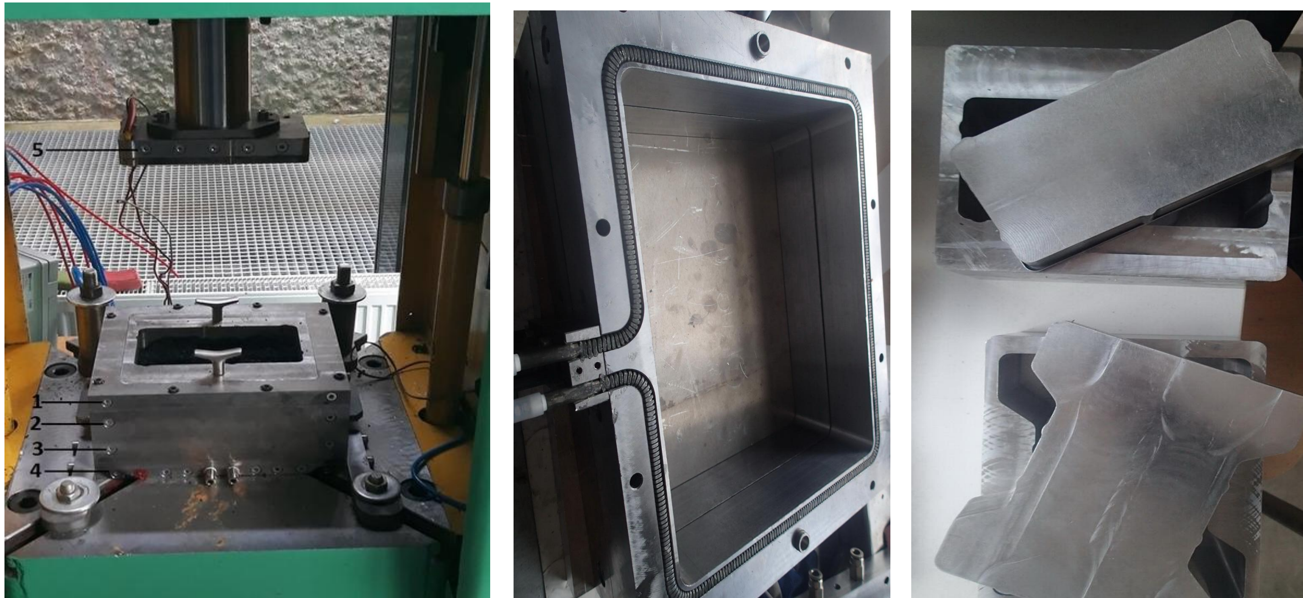
Fig.3. A view of the working area of the PHM-63h hydraulic press with the mould and punch fitted.
