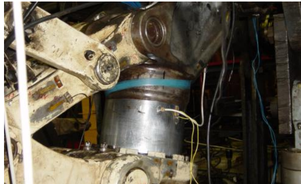
Fig. 4. Placement of a piezoelectric sensor and a strain gauge on the shock absorber rod mirror of an aircraft landing gear strut
