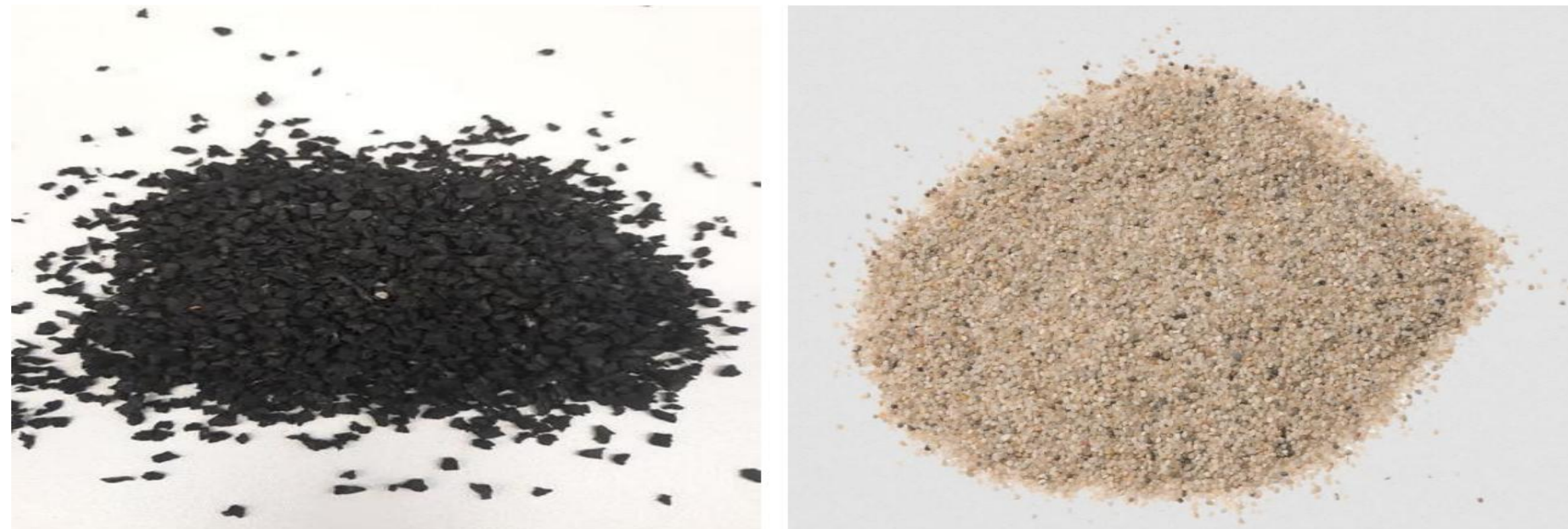
Fig.2. The EFDM-type rubber granules and mineral filler (quartz sand) used in the research.
